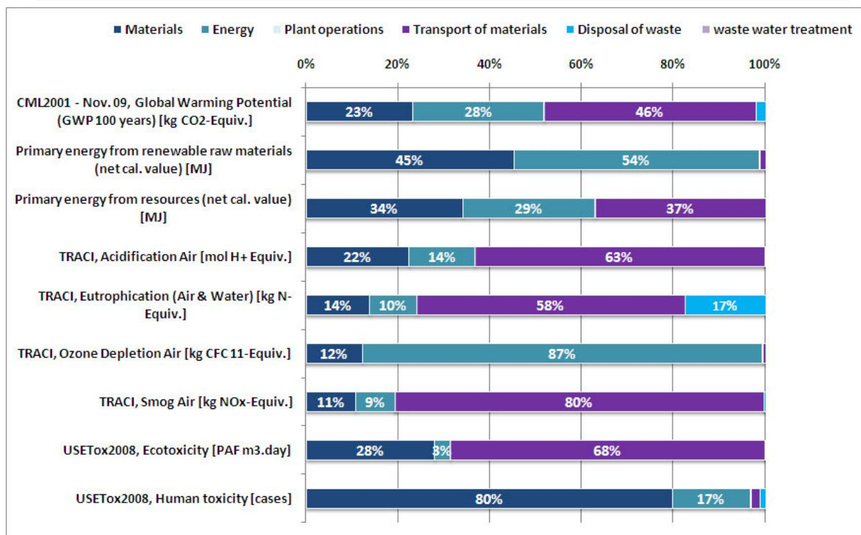
**Figure 6-6. Foil manufacturing for the cotton paper bank note (relative)**
