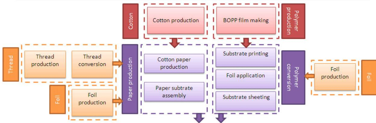
**Figure 4-7. Bank notes materials manufacturing phase model**
