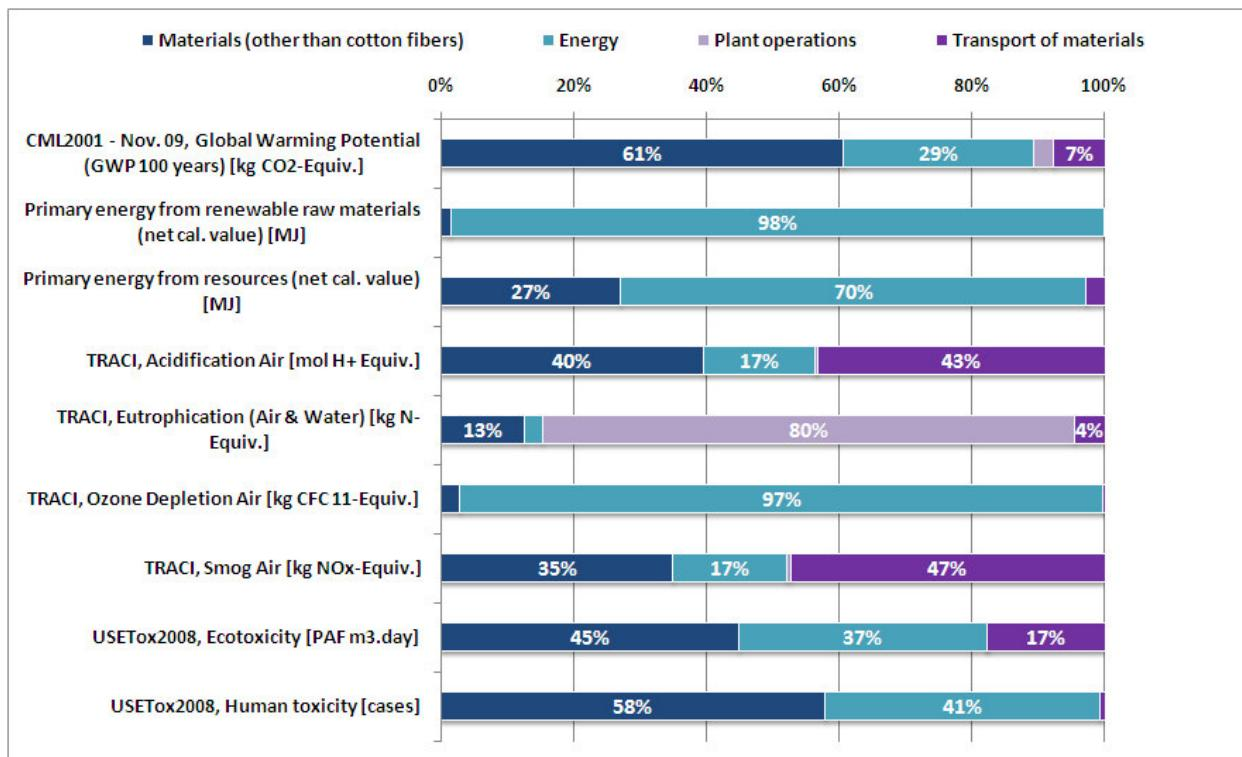
Figure 6-4. Cotton paper manufacturing (relative) – 100 bank notes, 2.5 manufacturing cycles
